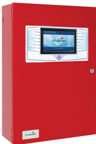
The base model of the FireNET L@titude Fire Alarm Control Panel is equipped with a generous quantity of notification appliance circuits, relays, and inputs, and can be further increased by the addition of up to four I/O panel modules.
